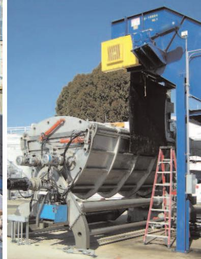
The DODA depackaging/preprocessing system at the Sacramento BioDigester is sized for a 100 tons/day. Loads include cans of off-spec food that are tipped onto the conveyor belt of the system.
