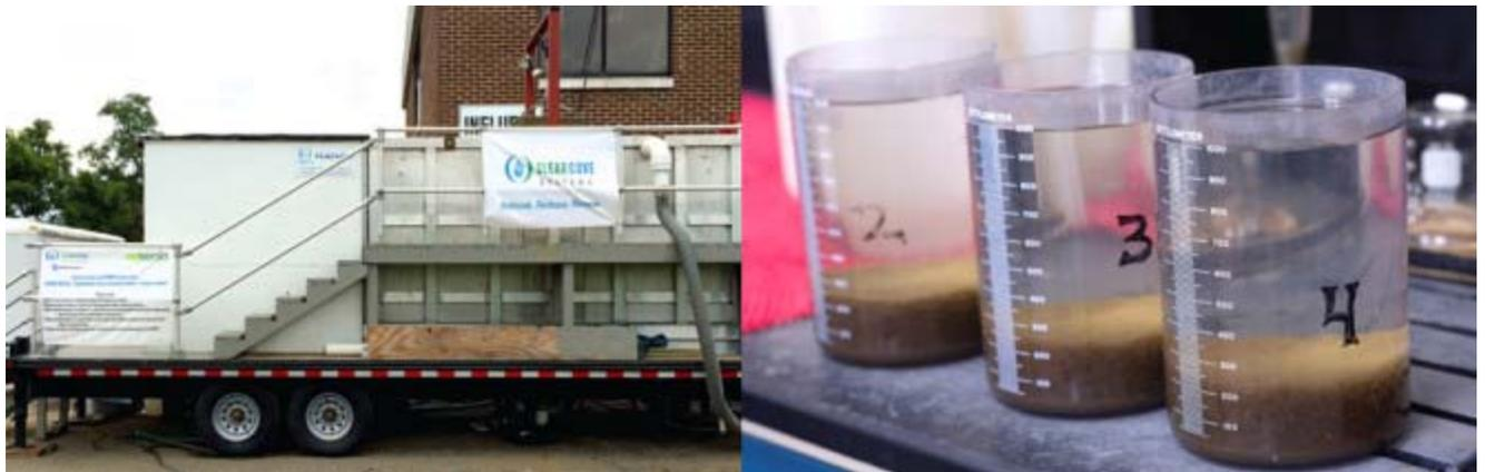
The ClearCove Enhanced Primary Treatment system was piloted at IAWWTF in 2014 (right). Organics and solids settle to the bottom of the tank, as illustrated in the samples at far right. Photo courtesy of A. Sue Weisler, RIT
